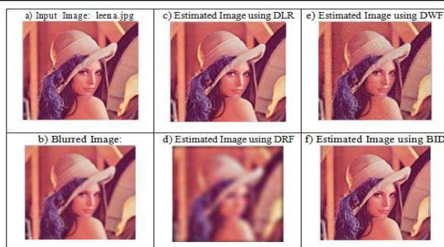
Fig. 5: Restoration Results for leena.jpg (256 x 256) blurred using a Gaussian Blur of size=5 and standard deviation=5
